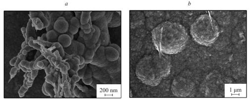
Fig. 3. The SEM image of Ni-MoO<sub>3</sub>:  $V_2O_5$  composite film: the initial stage of composite growing (a), the terminal stage of the composite growing (b)
