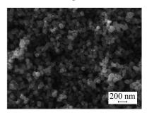
Fig. 5. XRD pattern (a) and SEM image (b) of a Fe NP sample prepared at 500 °C
