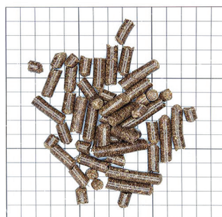
Fig. 1. Sedge pellets used for combustion experiments in Malchin [6]
