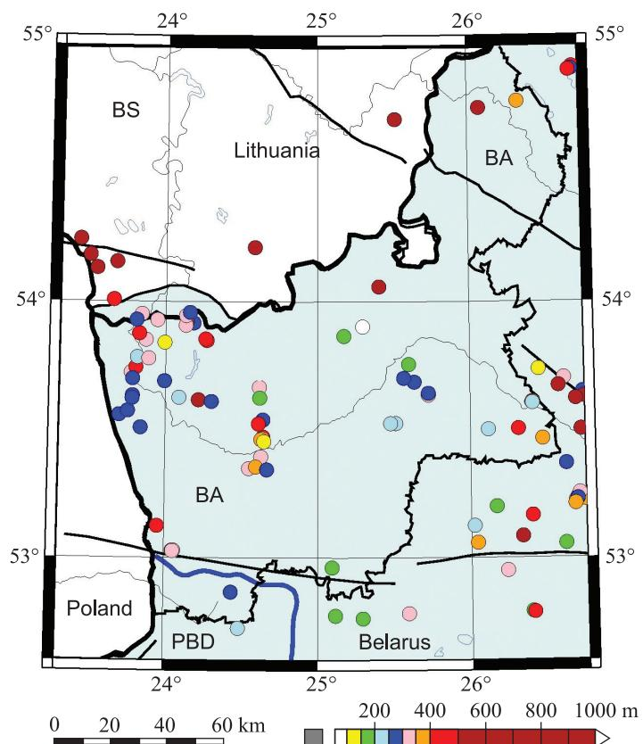
*Fig. 3.* Locations and depths of boreholes in the Grodno region with recorded thermograms.
