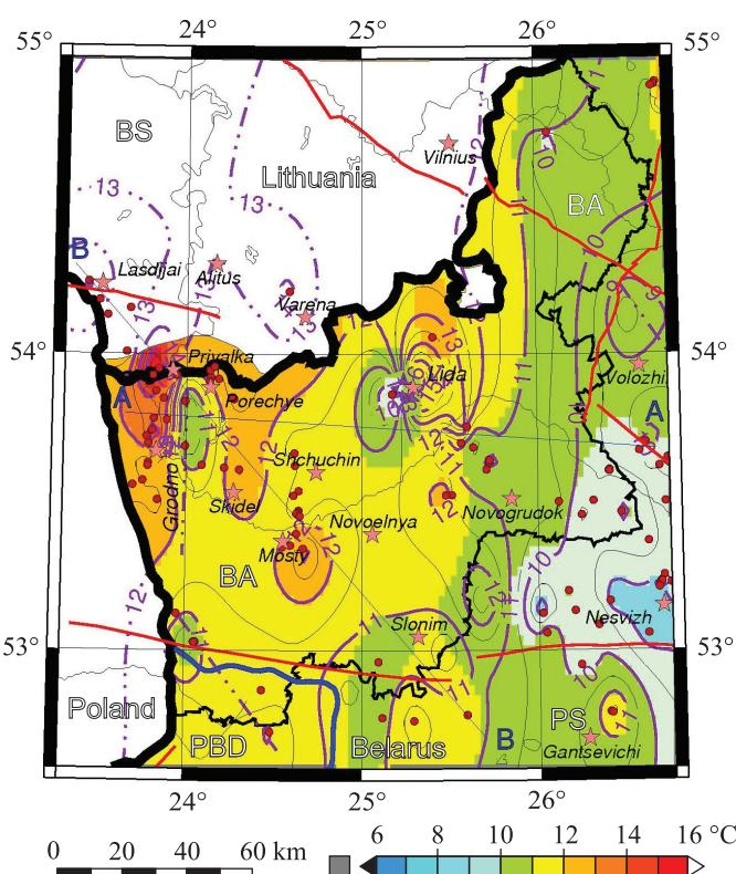
Fig. 9. Temperature distribution at 300 m depth within the Grodno region.
