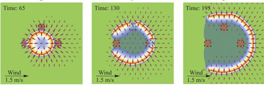
Fig. 7. Fire dynamics for the quadratic fuelbreak geometry at the following time points: 65 (a), 130 (b), 195 (c)
