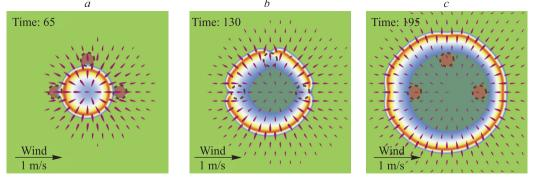
Fig. 9. Fire dynamics for the circular fuelbreaks at 1 m/s wind velocity at the following points: 65 (a), 130 (b), 195 (c)
