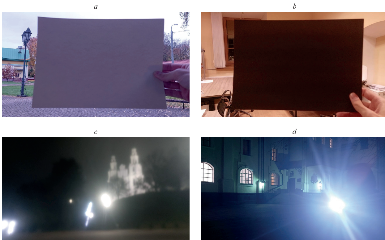
Fig. 5. Tampering scenarios for detector evaluation: a – covering the camera lens with a light-coloured object; b – covering the camera lens with a dark object; c – covering the camera lens with a translucent object; d – illuminating the lens with a bright light source
