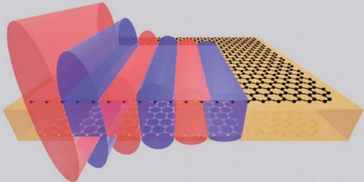
*Fig. 1.* Schematics of the considered system: the dielectric spacer with  $\epsilon_d$  in between of two graphene layers, surrounded by a media with the permittivity  $\epsilon_1 = 1$ . A propagating eigenmode is pictured schematically
