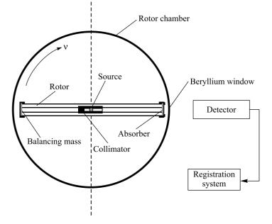
A typical scheme of the Mössbauer rotor experiment. The intensity of the resonant radiation passing resonant absorber is measured by the detector at the time moments, when the source, the absorber and the detector are aligned into a straight line. The thin iron-containing film of the resonant absorber is located inside beryllium shell of thickness of about 1 mm to prevent the absorber deformation due to centrifugal force
