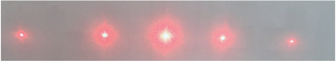
Fig. 7. Diffraction pattern on a relief-phase grating after the process of etching
