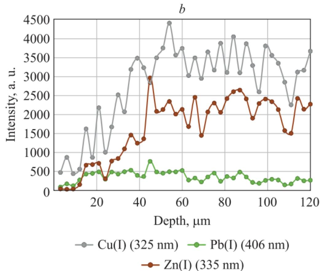
*Fig. 2.* Dependence of the relative intensity of the spectral lines of artifact components on the depth of laser ablation for a sample covered exclusively with patina (*a*) and scale (*b*)
