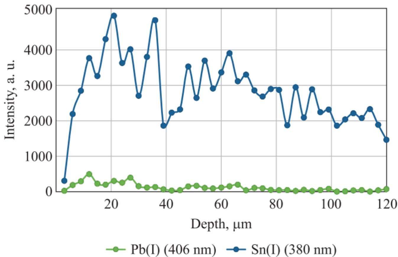
*Fig. 3.* The dependence of the relative intensity of the spectral lines of tin and lead on the depth of laser ablation for a product covered with a visible layer of scale
