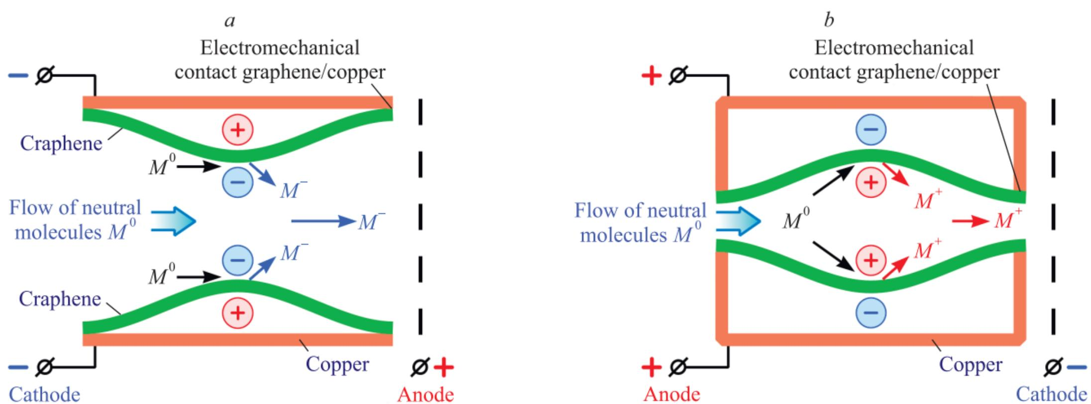
*Fig. 3.* Schemes for generation of a flow of molecular ions: *a* – scheme for generation of negative ions ( $M^-$ ) between convex graphene surfaces on a copper substrate (analogy of a Laval nozzle),  $WF(\varphi) < EA$ ;
