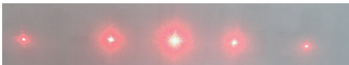
Fig. 7. Diffraction pattern on a relief-phase grating after the process of etching
