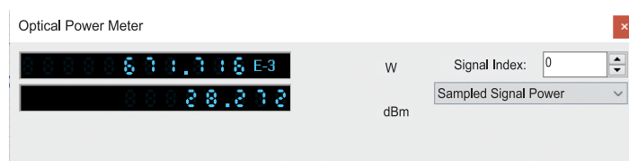
Fig. 7. Output power measured by the built in optical power meter ( Optisystem software)
